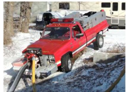
**The pickup with the front mount pump is used to fill tenders or as a relay truck. It set up by a river just down the street from the fire scene and was used to relay water to our attack engine as a supplement to the water supply we had set up. It is a very handy truck to have in a rural area!!**
