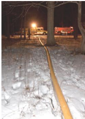
Above - the four sides of the structure. Below - LDH lead out from road into working engine was about 300'. Then laid was 100' up to the rear with a manifold. There were two engines pumping off road into fire scene.
